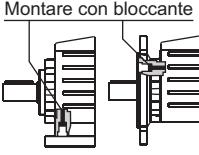
In applications where multiple starts, stops or reverses occurs, it is recommended to block the fastening bolts of the output flange and feet.
