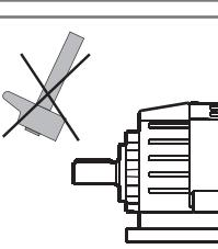
When mounting pinions, pulleys or couplings on the reducer's shaft, protect the bearings from impact by using the appropriate pullers and threaded holes in the end of the reducer shaft.
